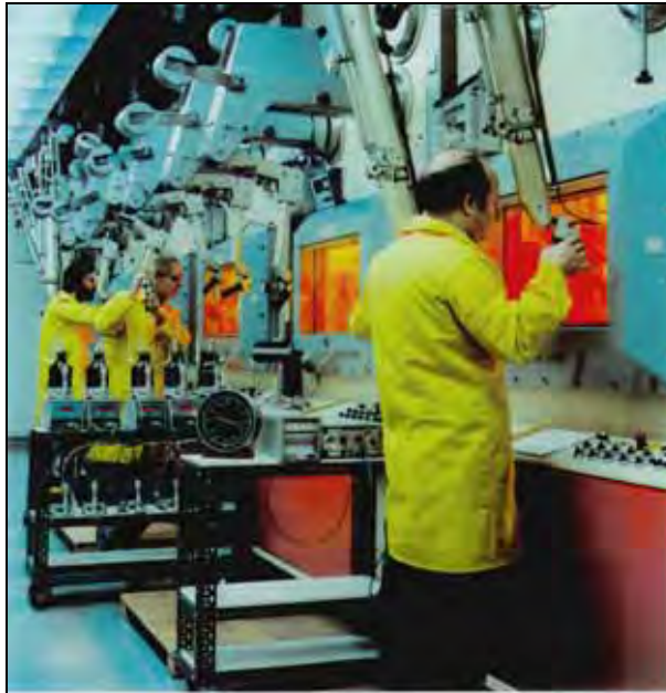
Hot cells, operator side with manipulators for remote-controlled work
