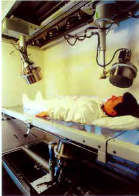
Body counter of the Research Centre Karlsruhe to determine the gamma-radiating radionuclides in the human body
