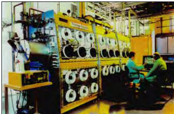
Laboratory for the handling of gaseous tritium in a row of glove boxes
